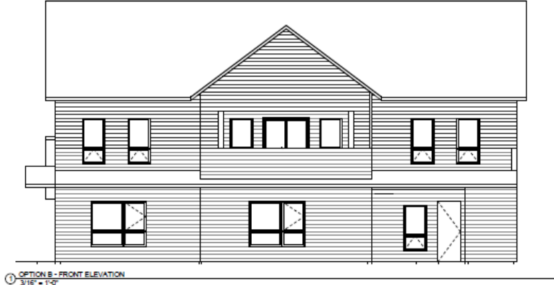
① OPTION B - FRONT ELEVATION 3/16" = 1'-0"
