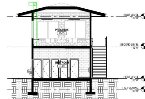
3 PRESENTATION SECTION - QUAD N/S SCALE: 1/8" = 1'-0"
