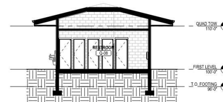
2 PRESENTATION SECTION - QUAD ALT N/S SCALE: 1/8" = 1'-0"
