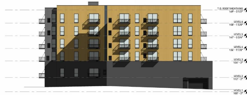
WEST EXTERIOR ELEVATION 1/16" = 1'-0"
