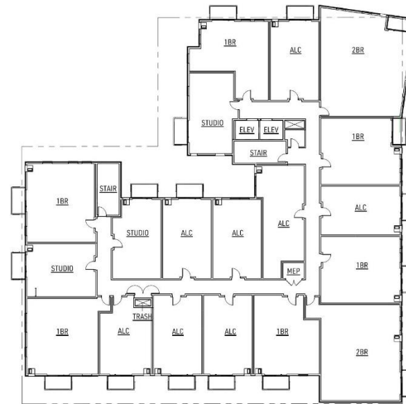
FLOOR PLAN - LEVELS 3-5 1/16" = 1'-0"
