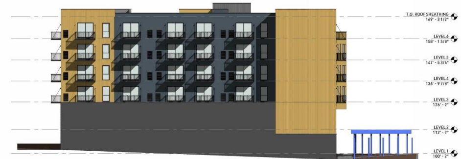
SOUTH EXTERIOR ELEVATION 1/16" = 1'-0"
