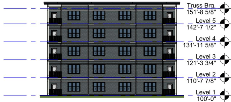
① Elevation - North End 3/64" = 1'-0"
